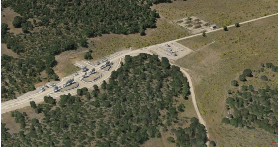
Figure 15. Training area of “Casas de Uceda”. 3D model from autocorrelation of photographic sensor images. CEGET Geodrone Mapper RTK RPAS system.
